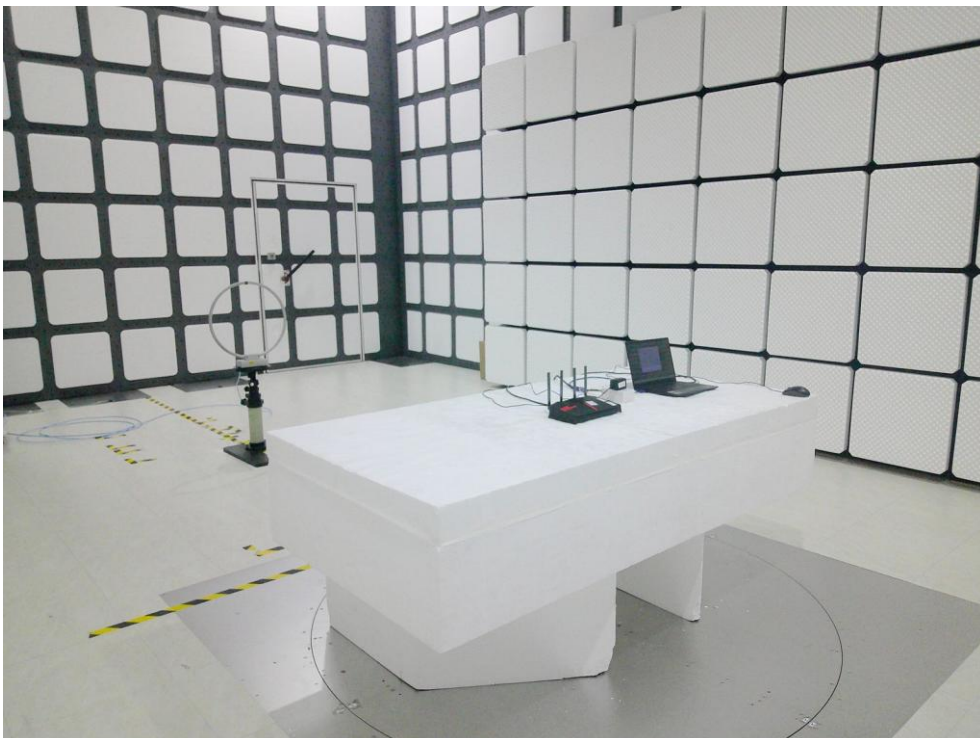
Description: Radiated Emission Test Setup for 9kHz~30MHz
