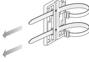
3. Fix the mounting bracket on the pole and fasten the strap, then secure the device into the mounting bracket as shown below.
