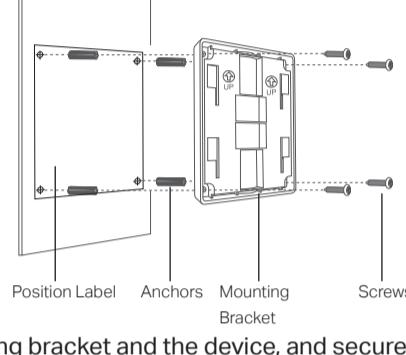
3. Align the mounting bracket and the device, and secure the device into the mounting bracket as shown below.
