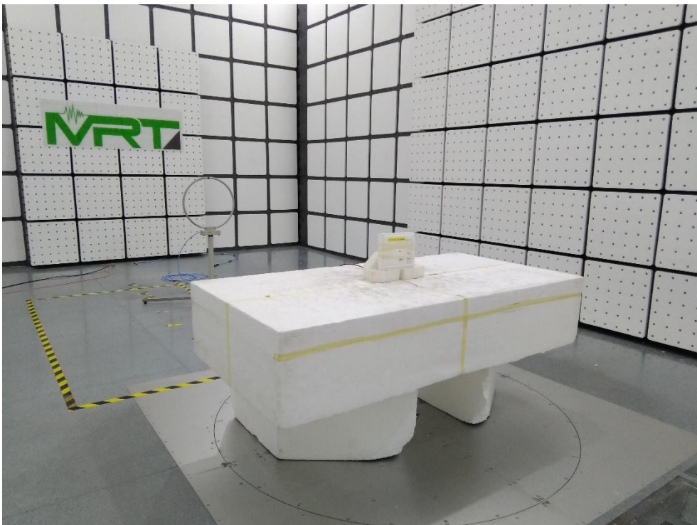
Description: Radiated Emission Test Setup for 9kHz~30MHz
