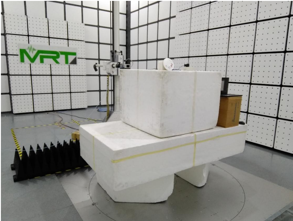
Description: Radiated Emission Test Setup for 9kHz~30MHz
