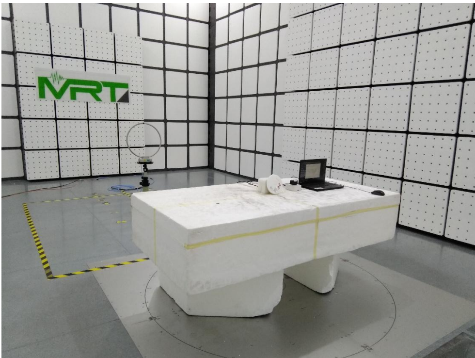
Description: Radiated Emission Test Setup for 9kHz~30MHz
