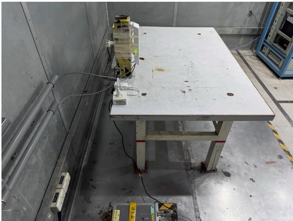
**Radiated Emissions Test Photos****9 kHz to 30 MHz**
