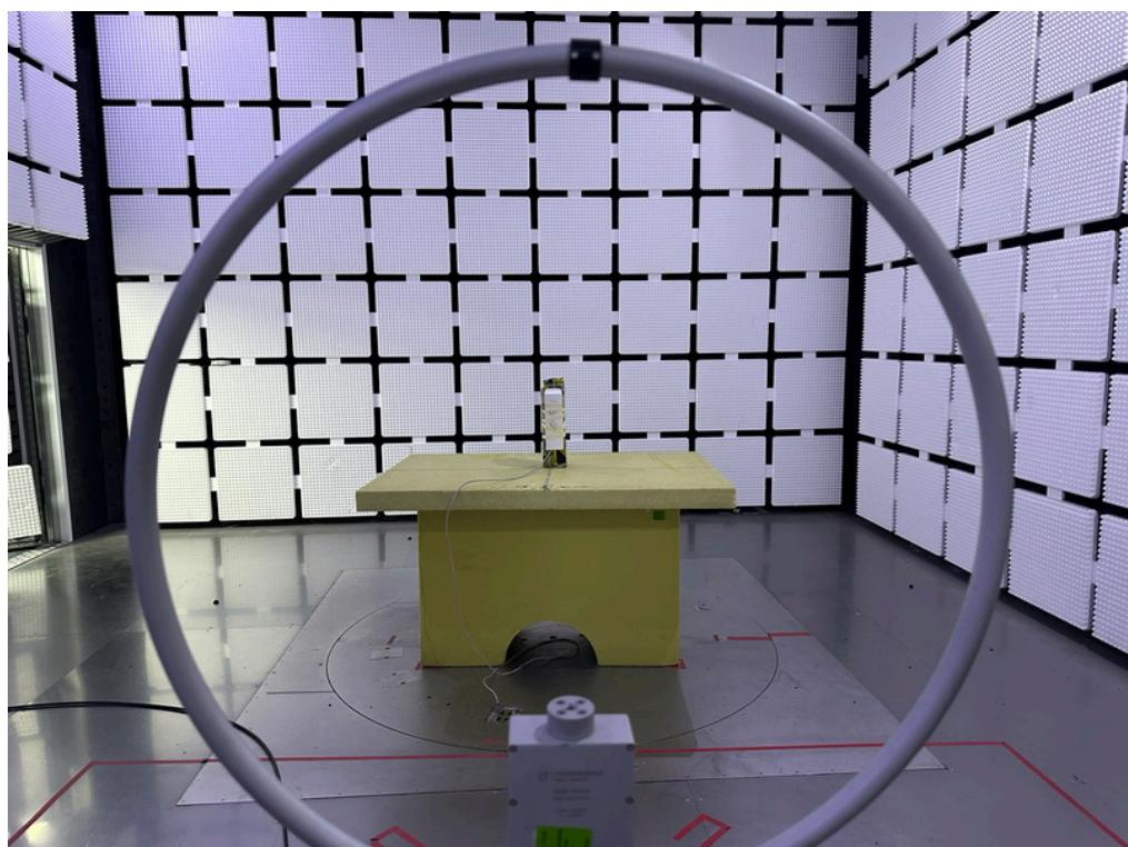
**Radiated Emissions Test Photos****30 MHz to 1 GHz**
