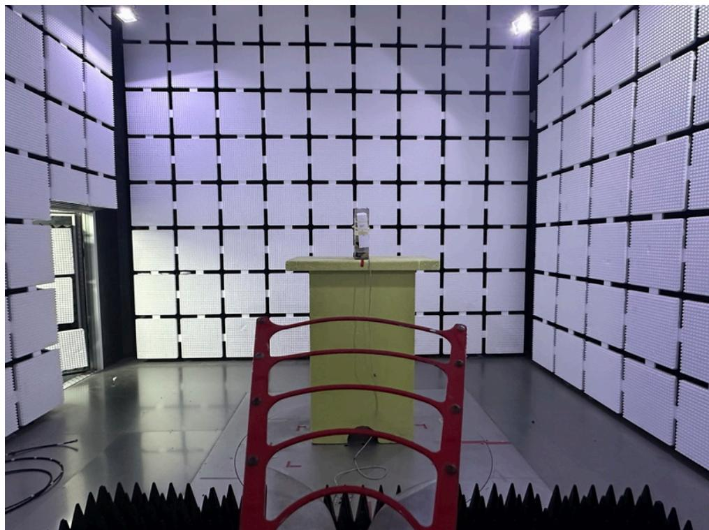
**Radiated Emissions Test Photos****Harmonic(18 GHz to 40 GHz)**
