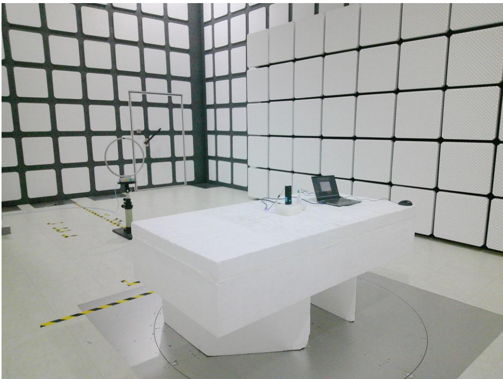
Description: Radiated Emission Test Setup for 9kHz~30MHz
