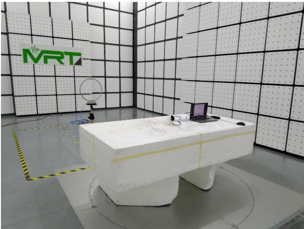
Description: Radiated Emission Test Setup for 9kHz~30MHz
