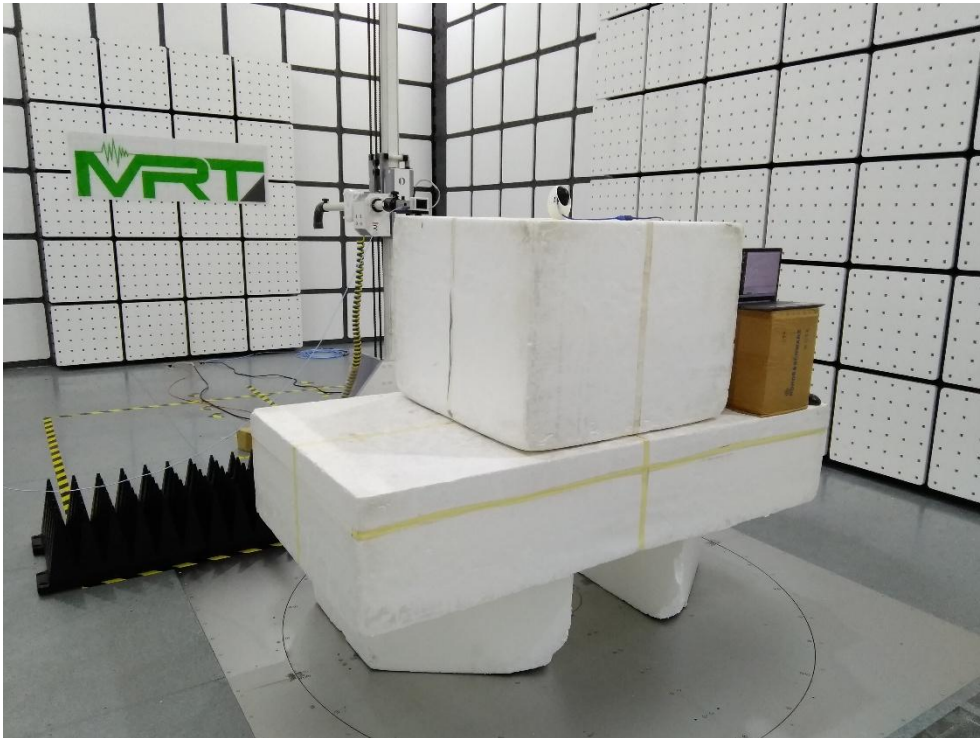
Description: Radiated Emission Test Setup for 9kHz~30MHz
