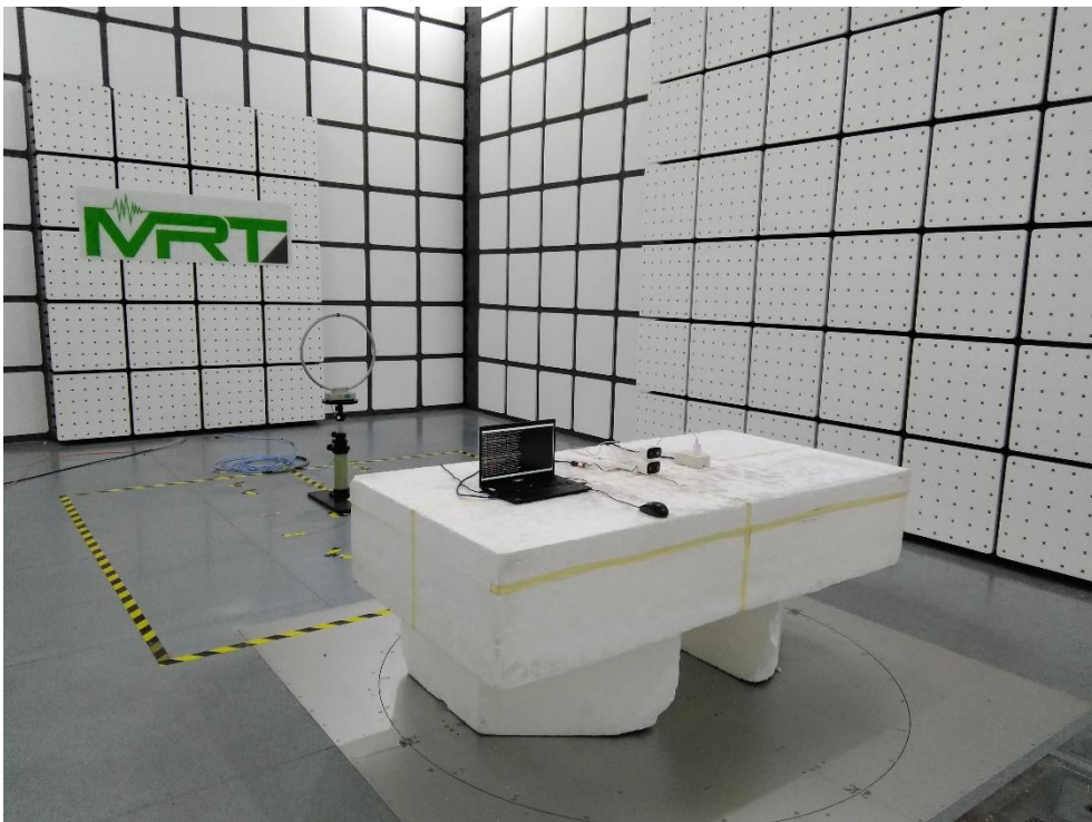
Description: Radiated Emission Test Setup for 9kHz~30MHz
