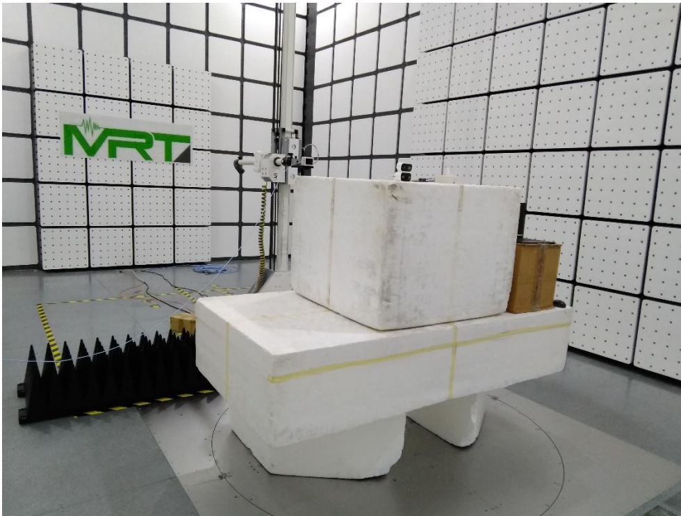
Description: Radiated Emission Test Setup for 9kHz~30MHz
