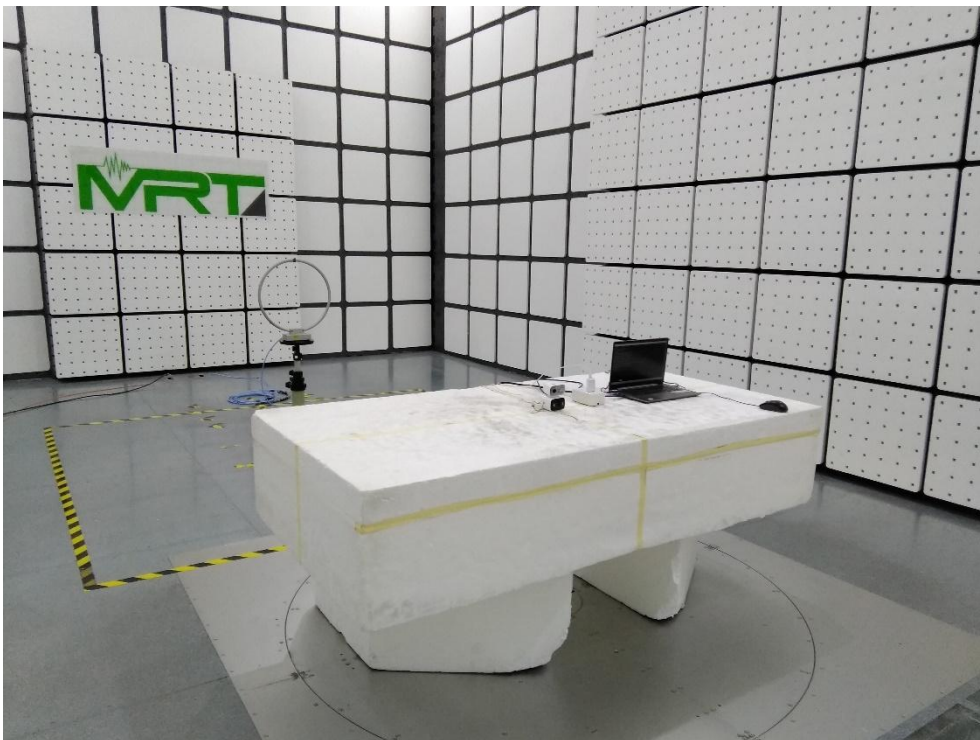
Description: Radiated Emission Test Setup for 9kHz~30MHz
