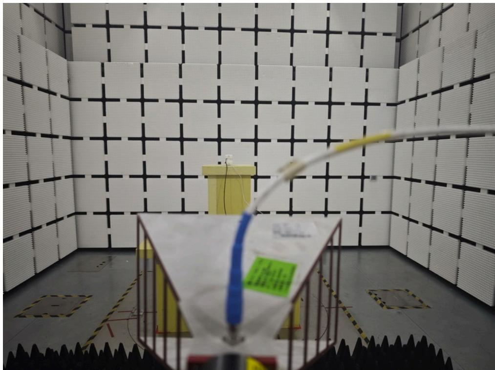
**Radiated Emissions Test Photos****Harmonic(18 GHz to 26.5 GHz)**
