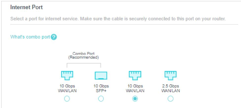
1. Select the desired internet port. Make sure the cable is securely connected to this port on your router.
