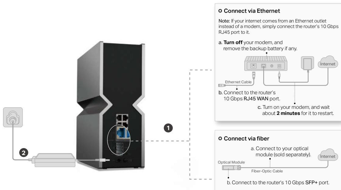
2. Connect the power adapter to the router and turn on the router.
