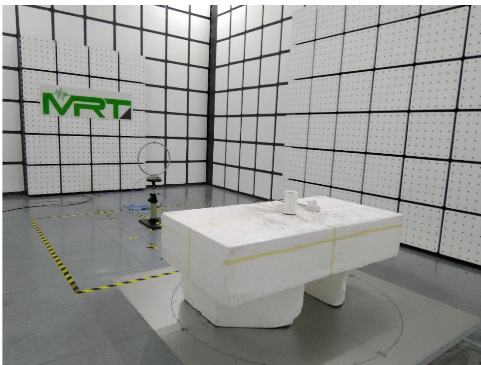
Description: Radiated Emission Test Setup for 9kHz~30MHz
