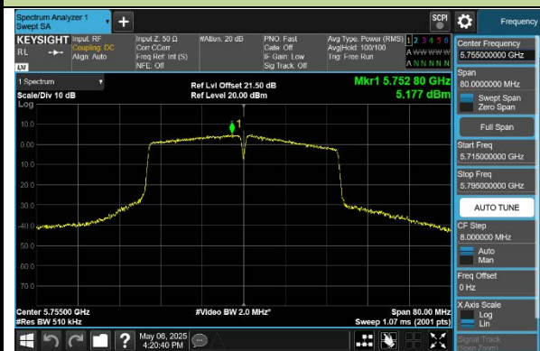
802.11ac-VHT80 Power Spectral Density - Ant 0
