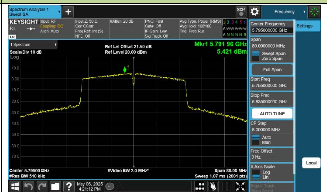
802.11ac-VHT80 Power Spectral Density - Ant 0
