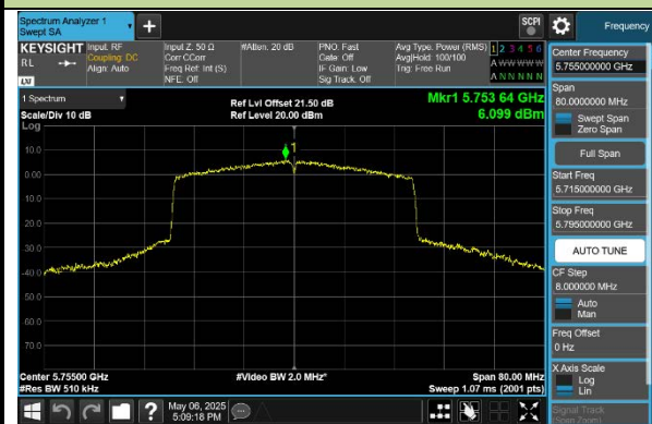
802.11ax-HE80 Power Spectral Density - Ant 0
