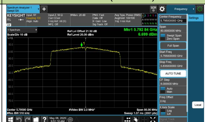
802.11ax-HE80 Power Spectral Density - Ant 0
