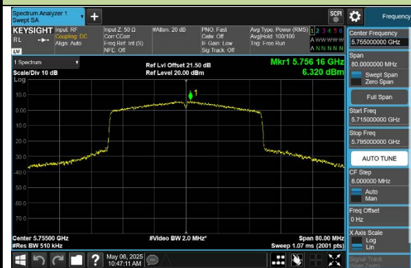
802.11ac-VHT80 Power Spectral Density - Ant 0
