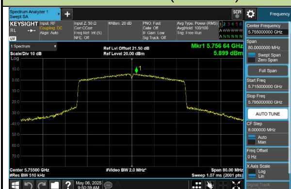
802.11ax-HE80 Power Spectral Density - Ant 0
