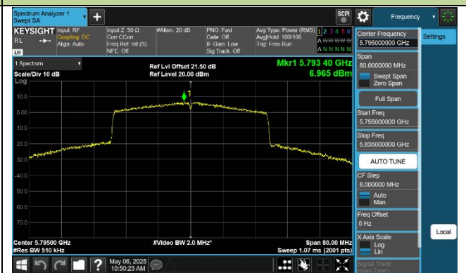
802.11ac-VHT80 Power Spectral Density - Ant 0
