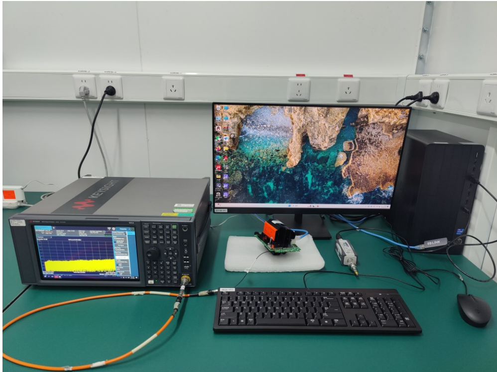
Description: Contention Based Protocol Measurement Test Setup for AP Mode
