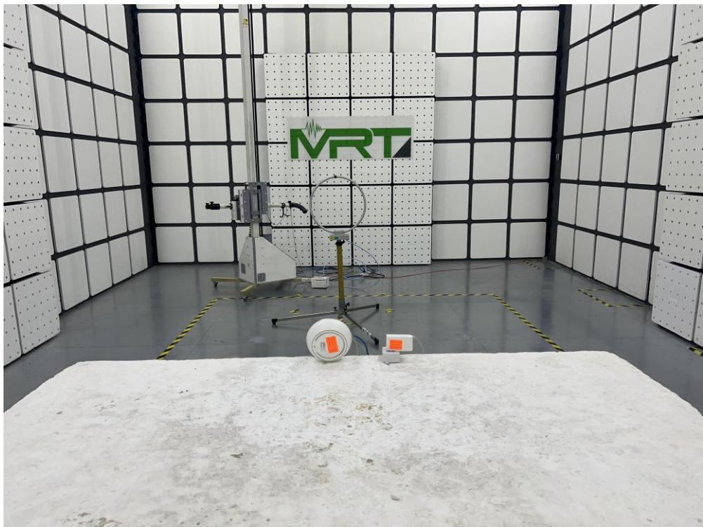
Description: Radiated Spurious Emissions Test Setup for 30MHz ~ 1GHz
