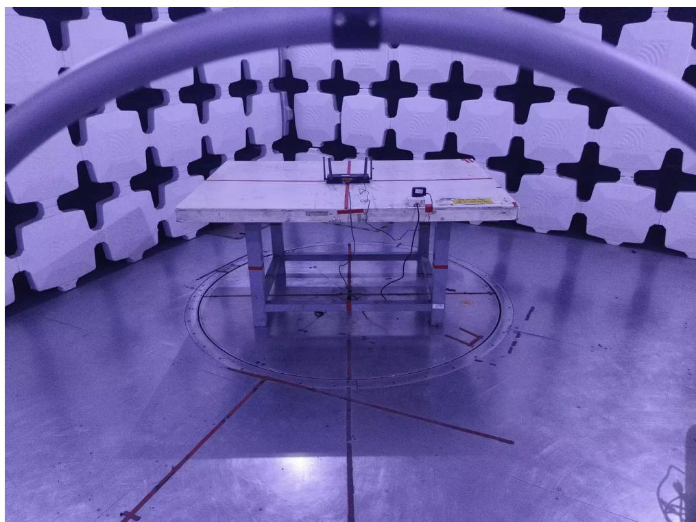
**Radiated Emissions Test Photos****30 MHz to 1 GHz**
