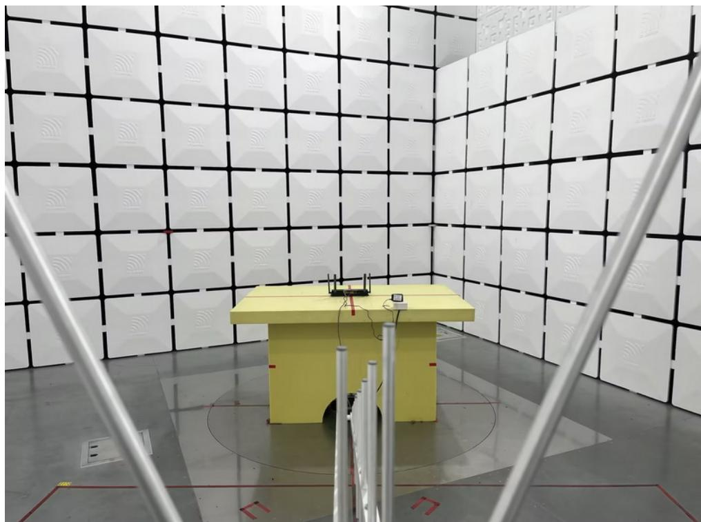
**Radiated Emissions Test Photos****1 GHz to 18 GHz**
