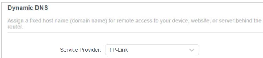
The screenshot shows a configuration page for Dynamic DNS. At the top, it says "Dynamic DNS" and provides a brief description: "Assign a fixed host name (domain name) for remote access to your device, website, or server behind the router." Below this, there is a "Service Provider" dropdown menu with "TP-Link" selected. The dropdown has a small downward arrow icon to its right.
