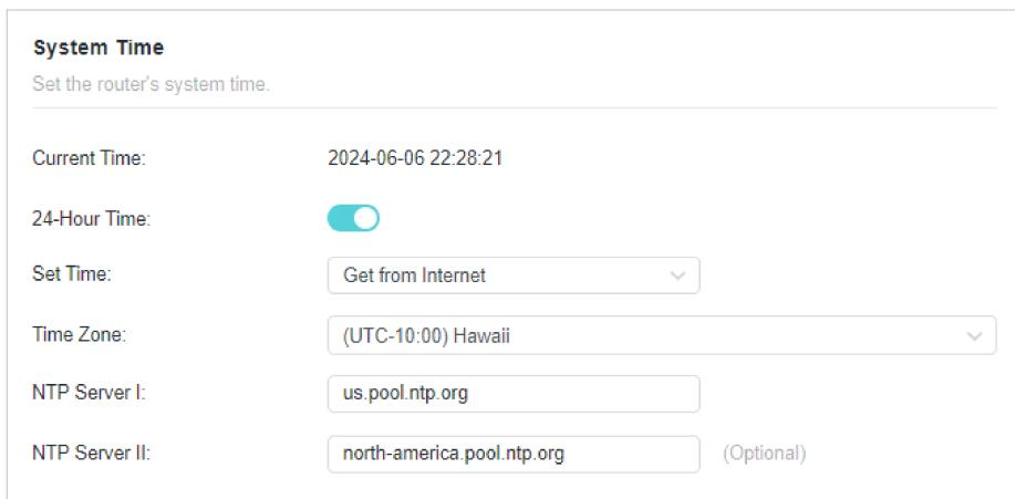
The screenshot shows the 'System Time' configuration page. The 'Set Time' dropdown is set to 'Get from Internet'. The 'Time Zone' dropdown is set to '(UTC-10:00) Hawaii'. The 'NTP Server I' field contains 'us.pool.ntp.org'. The 'NTP Server II' field contains 'north-america.pool.ntp.org' with '(Optional)' text next to it.
