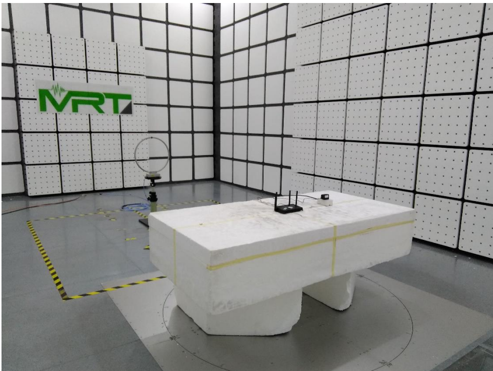
Description: Radiated Emission Test Setup for 9kHz~30MHz
