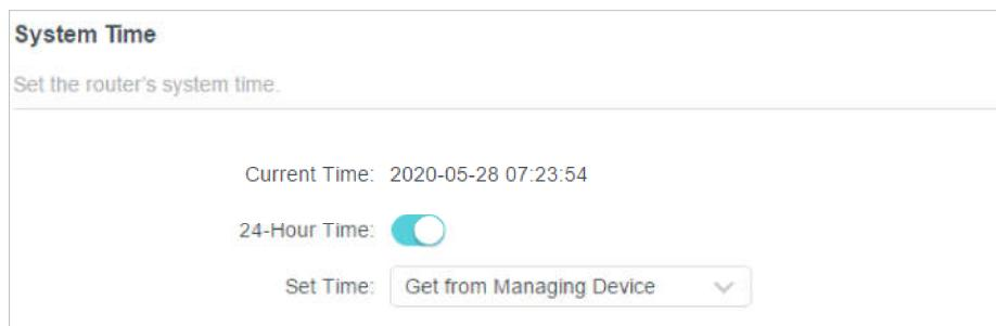
The screenshot shows the 'System Time' configuration page. The 'Set Time' dropdown is set to 'Get from Managing Device'. The current time is displayed as 2020-05-28 07:23:54, and the '24-Hour Time' switch is turned on.
