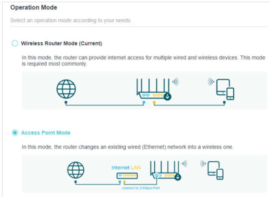
3. After rebooting, connect the router to your existing wired router via an Ethernet cable.
