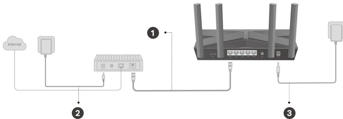
1. Connect the **powered-off modem** to the router's **WAN port** with an Ethernet cable.
