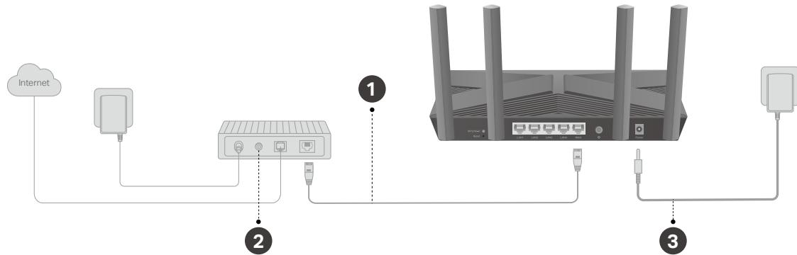
1. Connect the **powered-off modem** to the router's **WAN port** with an Ethernet cable.
