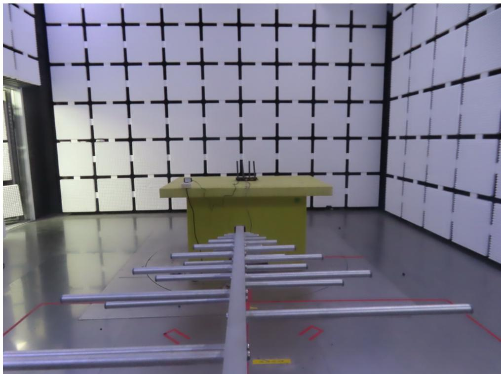
**Radiated Emissions Test Photos****Band edge & Harmonic(1 GHz to 18 GHz)**
