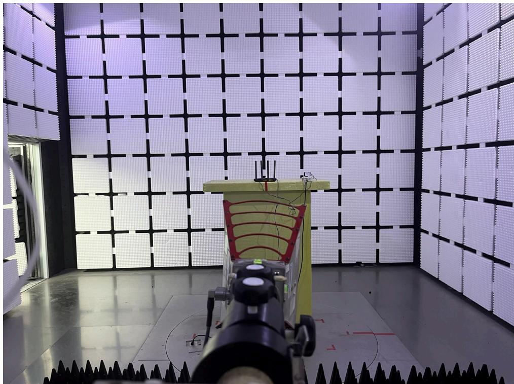
**Radiated Emissions Test Photos****Harmonic(18 GHz to 26.5 GHz)**
