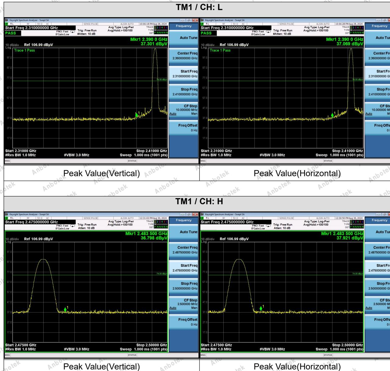
Note: When the PK measure result value is less than the AVG limit value, the AV measure result values test not applicable.
