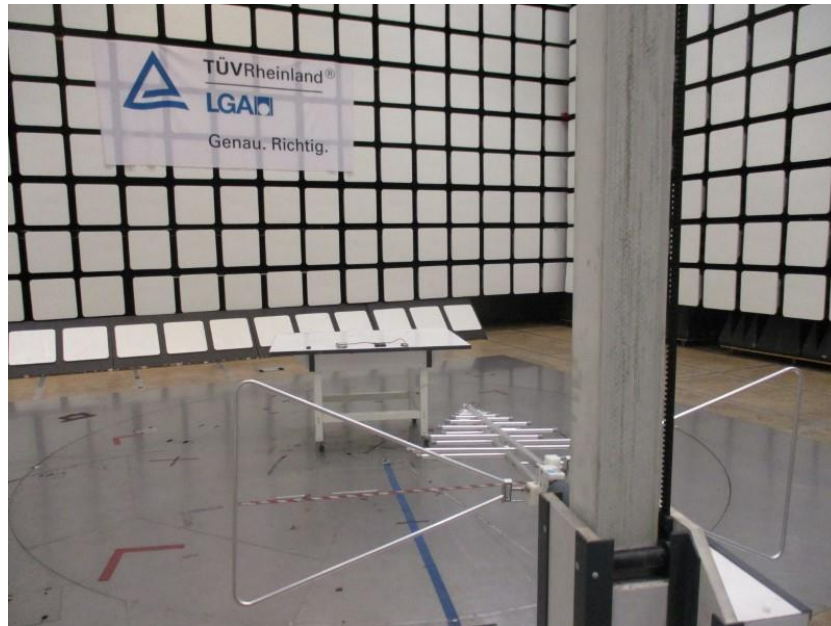
Picture 1: Radiated disturbance 30M-1GHz
