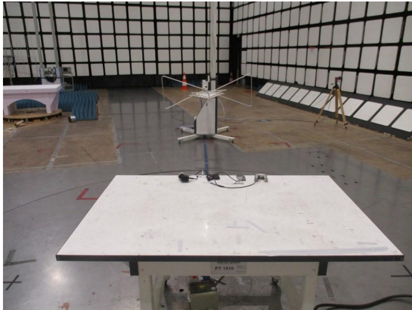
Picture 3: Radiated disturbance 30M-1GHz
