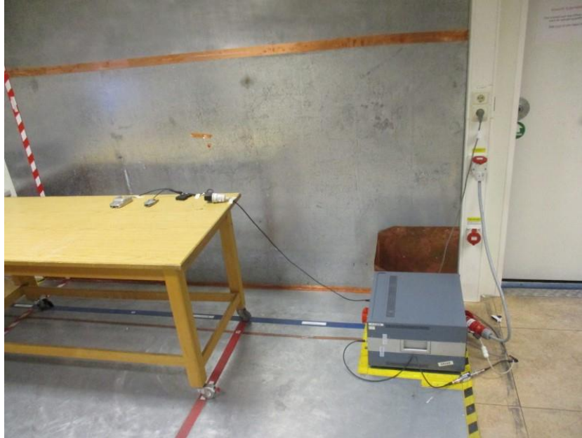
Picture 7: Conducted voltage emissions on AC Supply line
