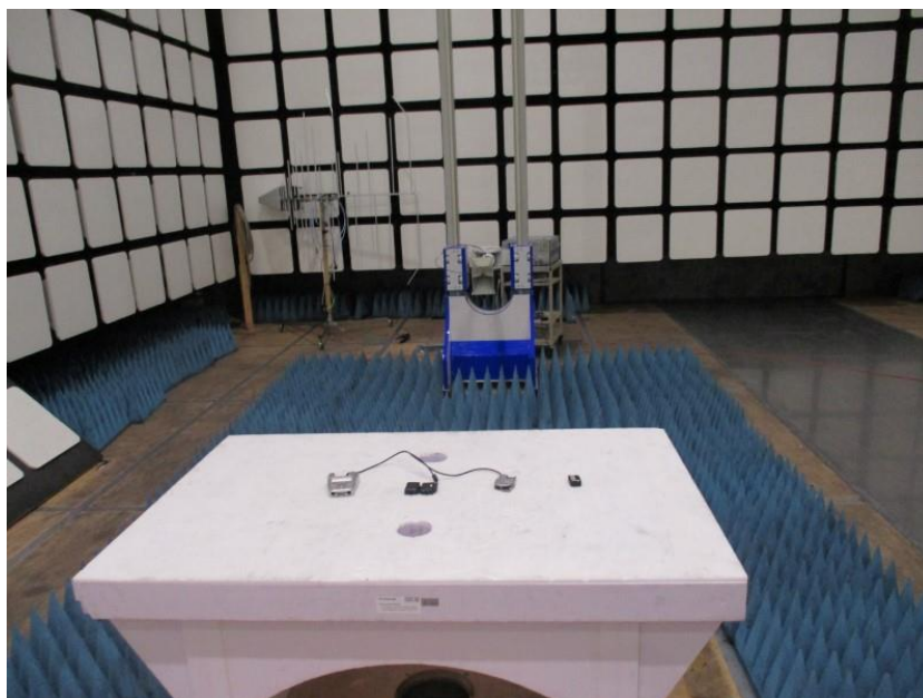
Picture 6: Radiated disturbance >1GHz
