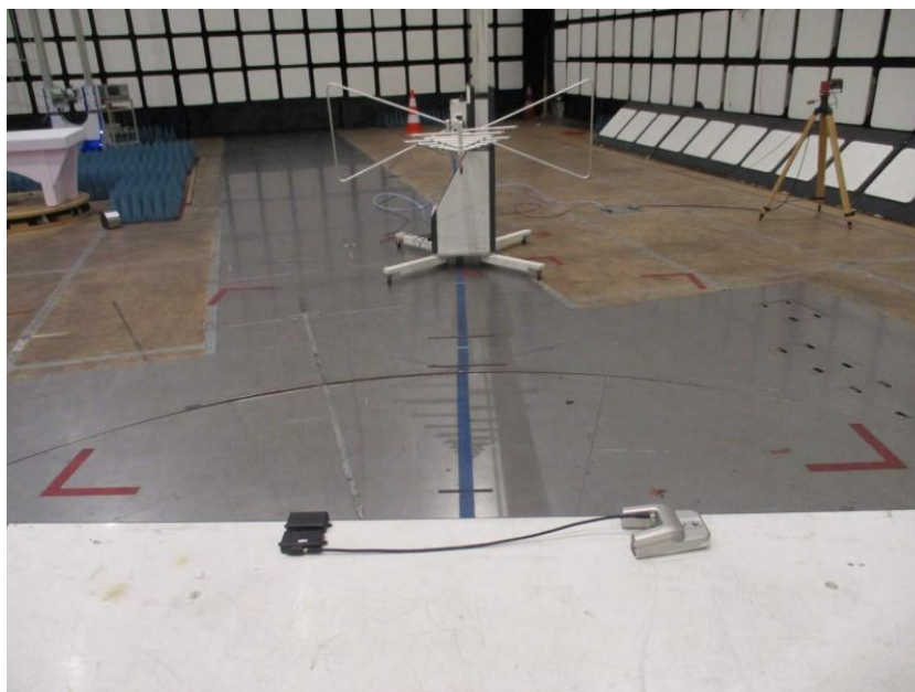
Picture 4: Radiated disturbance 30M-1GHz (see test protocol 52, test with alternative setup just for information)
