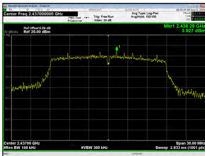
Tx. Spurious NVNT n20 2437MHz Ant1 Emission
