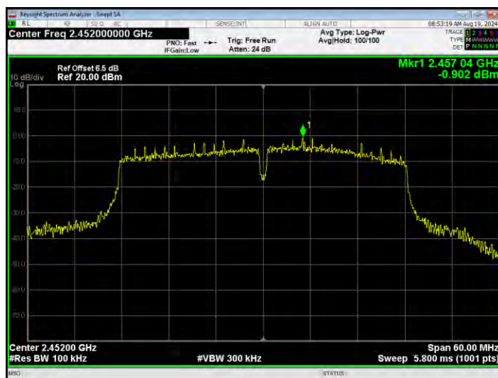
Tx. Spurious NVNT n40 2452MHz Ant1 Emission
