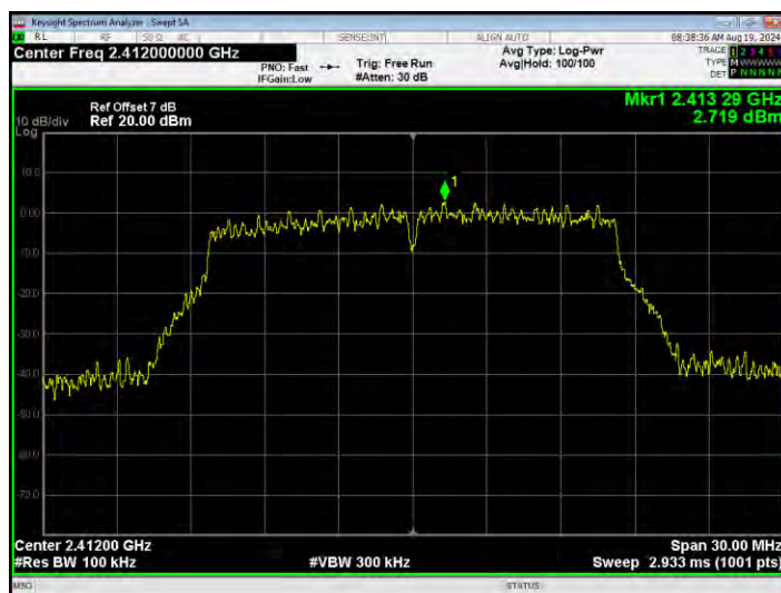
Band Edge NVNT g 2412MHz Ant1 Emission
