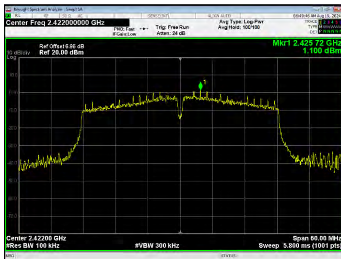
Tx. Spurious NVNT n40 2422MHz Ant1 Emission
