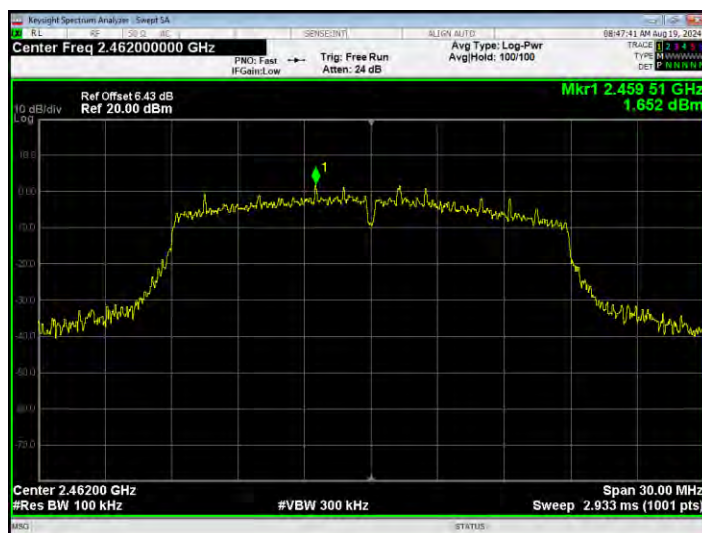
Band Edge NVNT n20 2462MHz Ant1 Emission
