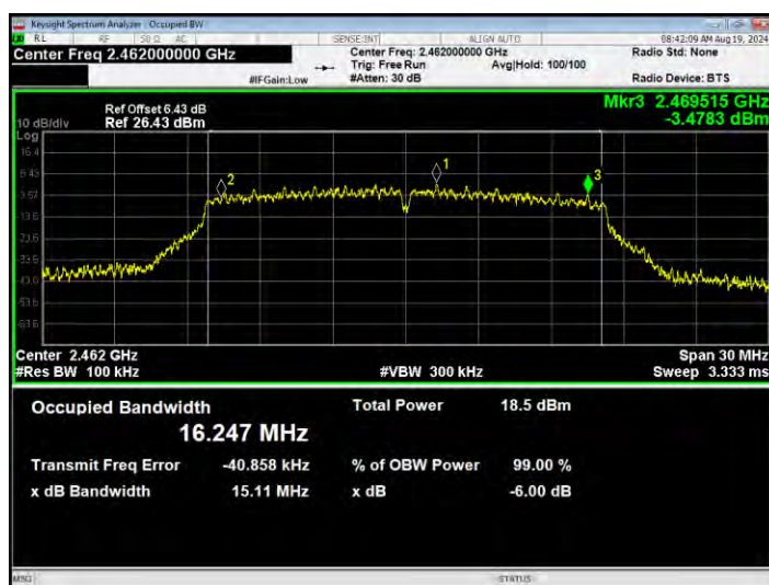
-6dB Bandwidth NVNT n20 2412MHz Ant1
