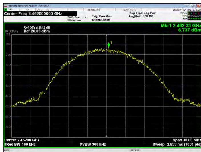
Band Edge NVNT b 2462MHz Ant1 Emission
