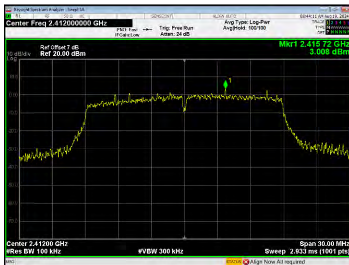
Tx. Spurious NVNT n20 2412MHz Ant1 Emission
