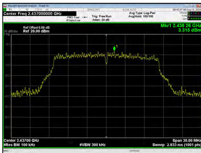
Tx. Spurious NVNT g 2437MHz Ant1 Emission
