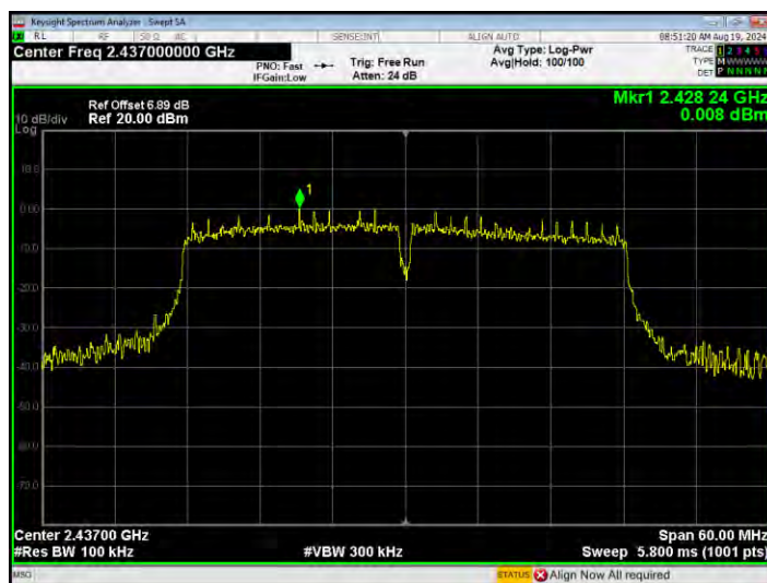
Tx. Spurious NVNT n40 2437MHz Ant1 Emission
