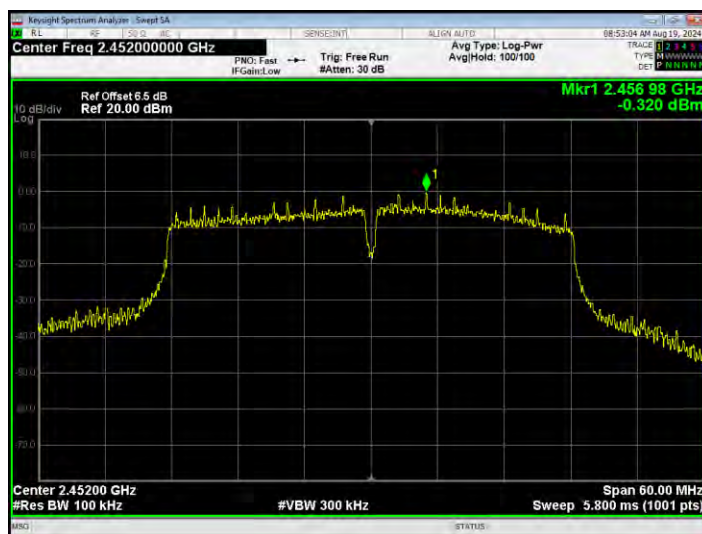
Band Edge NVNT n40 2452MHz Ant1 Emission
