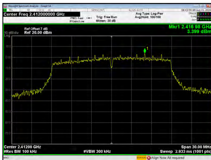
Band Edge NVNT n20 2412MHz Ant1 Emission
