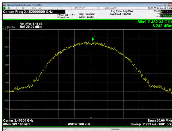
Tx. Spurious NVNT b 2462MHz Ant1 Emission
