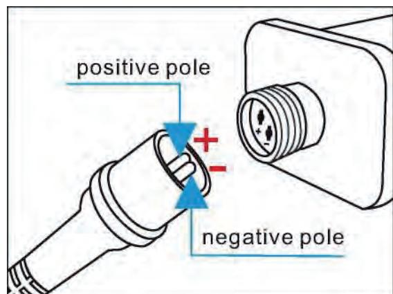
The connection between the controller and the power supply
