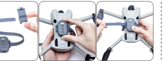
1. Secure the alarm to the top of the drone.
