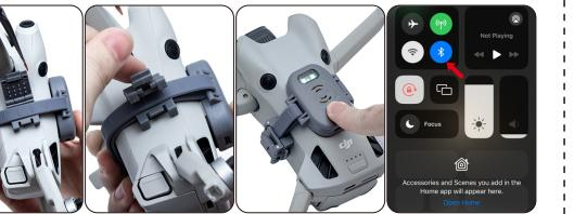
3. The strap fastener can be moved along the silicone strap to adjust its position according to different drone models.
