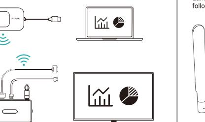
1. Connect the HD port or VGA port of the receiver to the video input port of the display device such as the monitor or TV.
