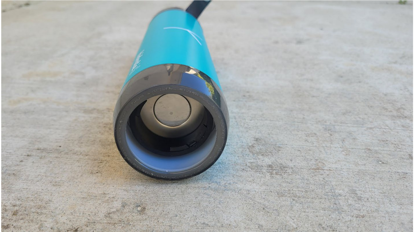
Bottom View of the Water Bottle (Sensor 007 screws into bottom)
