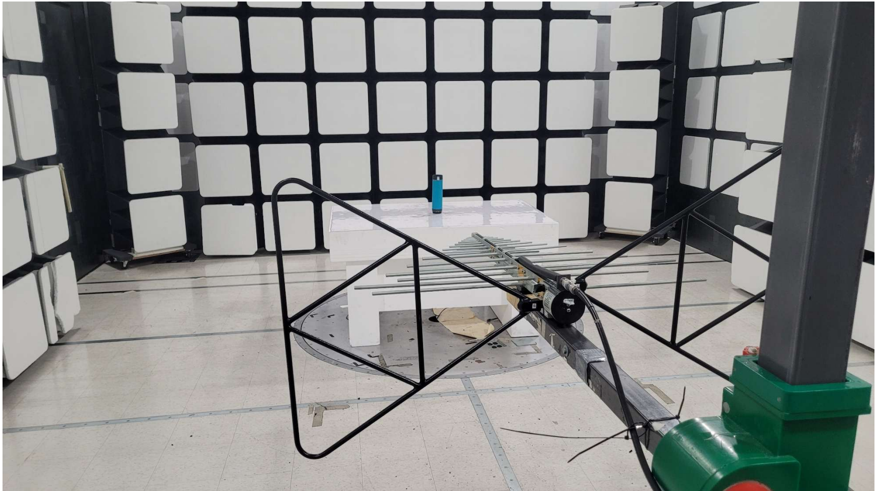
Normal Mode Radiated Emission
