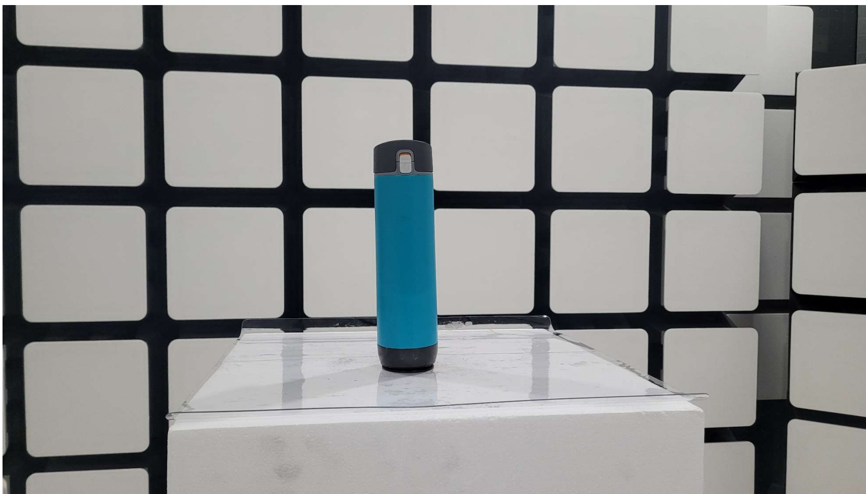
Normal Mode Radiated Emission Close Up
