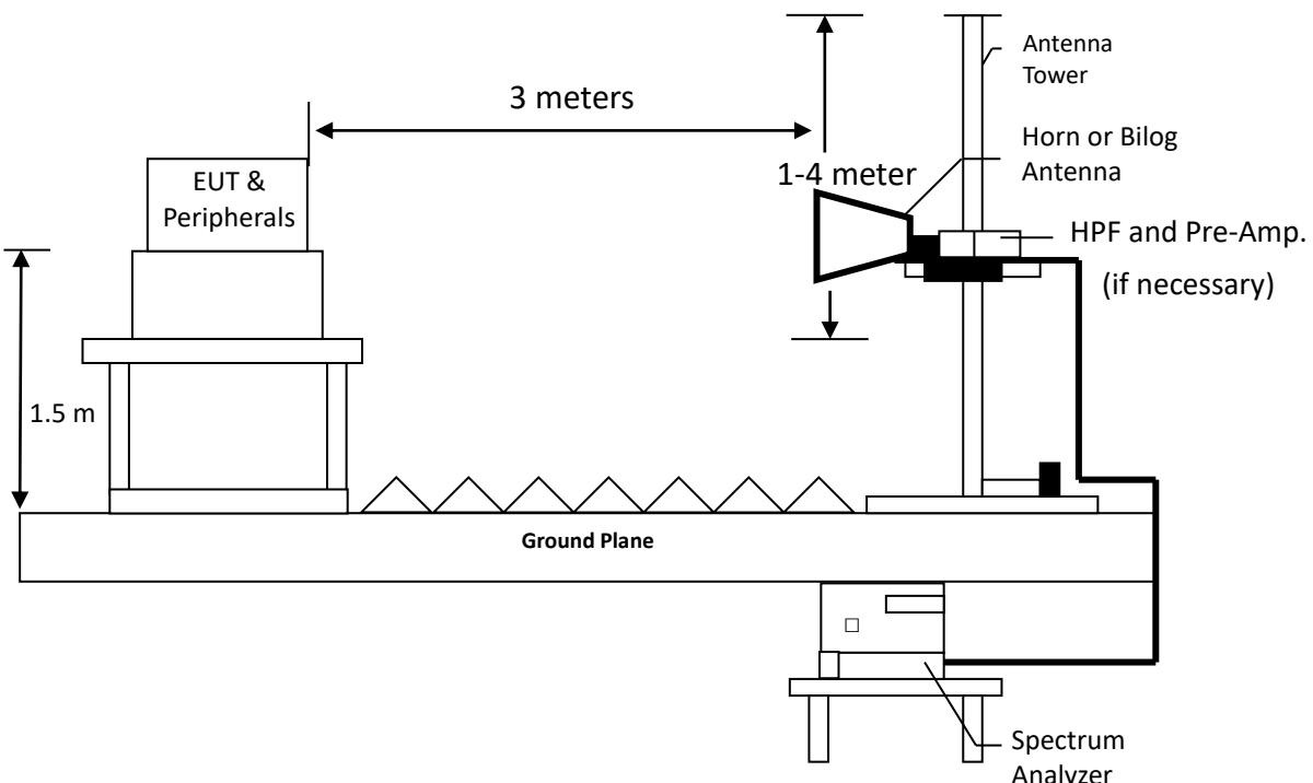
Radiated emissions were investigated cover the frequency range from 30MHz to 1000MHz using a receiver RBW of 120kHz record QP reading, and the frequency over 1GHz using a spectrum analyzer RBW of 1MHz and 10Hz VBW record Average reading. (15.209 paragraph), the Peak reading (1 MHz RBW/ 3 MHz VBW) recorded also on the report.
