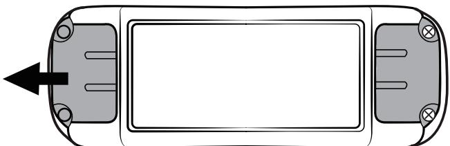
3. You can screw the wire on the terminal now after taking off cover
