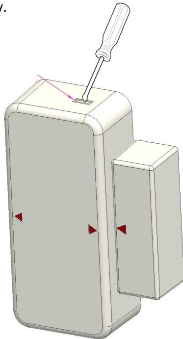
Press and hold "RF Connect" for 5 seconds to enter pairing mode.
