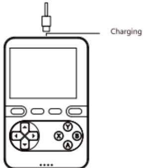
In addition, you can use any other proper available USB-compatible DC adapter to supply power from the power outlet. after the connection completes .press the power switch on the back of the mobile (figure1) to start game machine.
