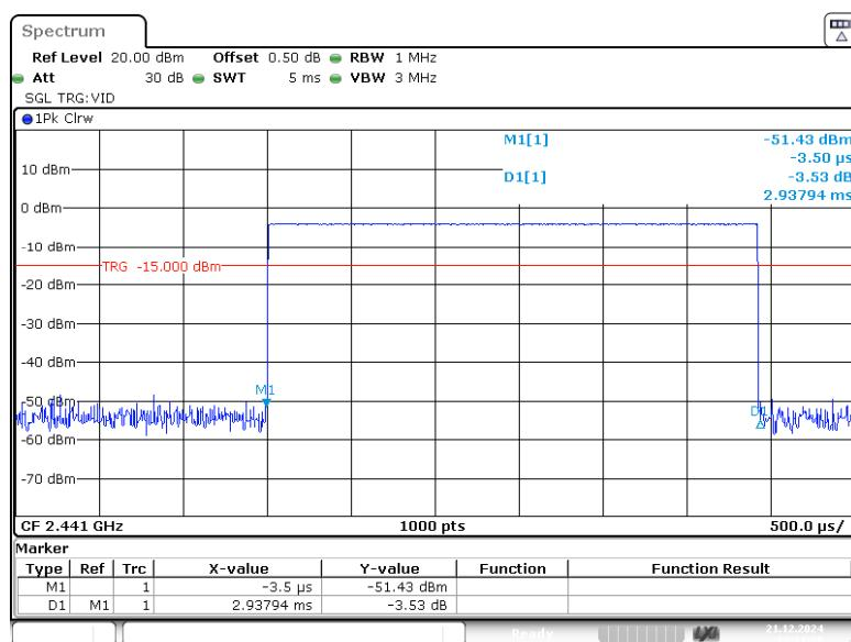
EDR ( $\pi/4$ -DQPSK)\_Hopping\_2DH1
