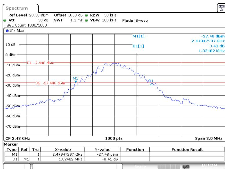
EDR ( $\pi/4$ -DQPSK): Low Channel
