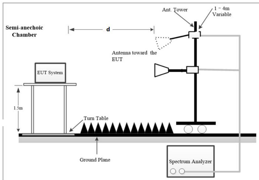
The radiated emission tests using the setup accordance with the ANSI C63.10-2013. The specification used was the FCC 15.209, FCC 15.247, RSS-247, RSS-Gen limits.
