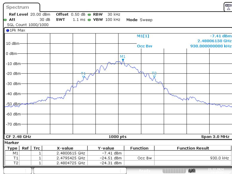
EDR ( $\pi/4$ -DQPSK): Low Channel
