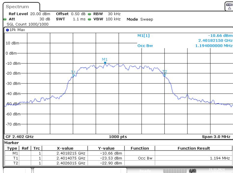
EDR ( $\pi/4$ -DQPSK): Middle Channel
