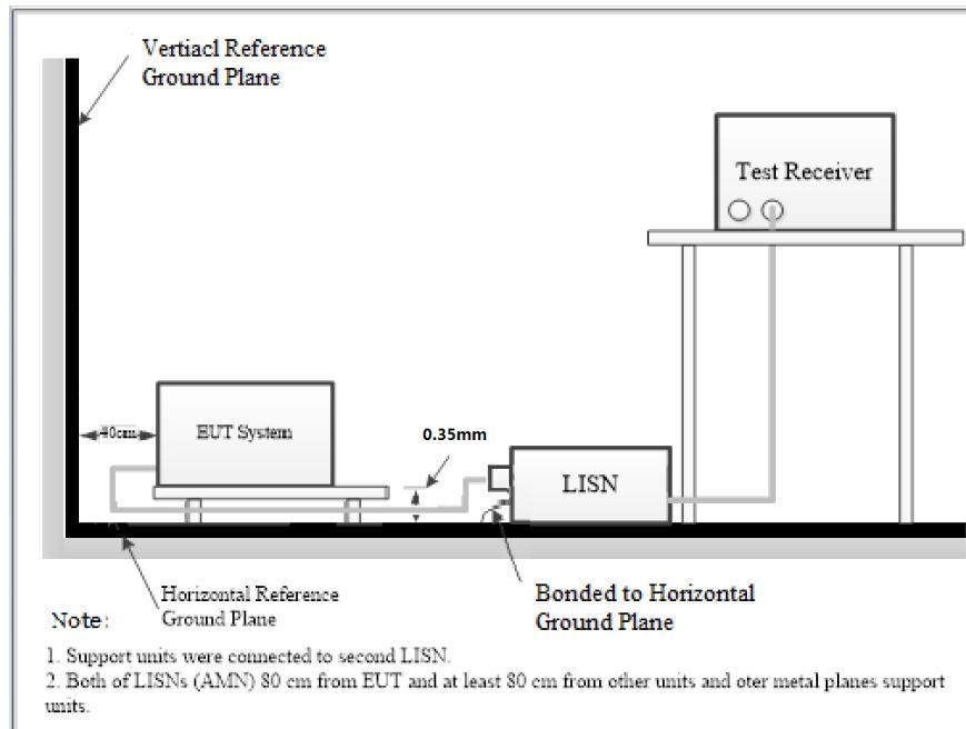
The measurement procedure of EUT setup is according with ANSI C63.10-2013. The related limit was specified in FCC Part 15.207, RSS-Gen limits.
