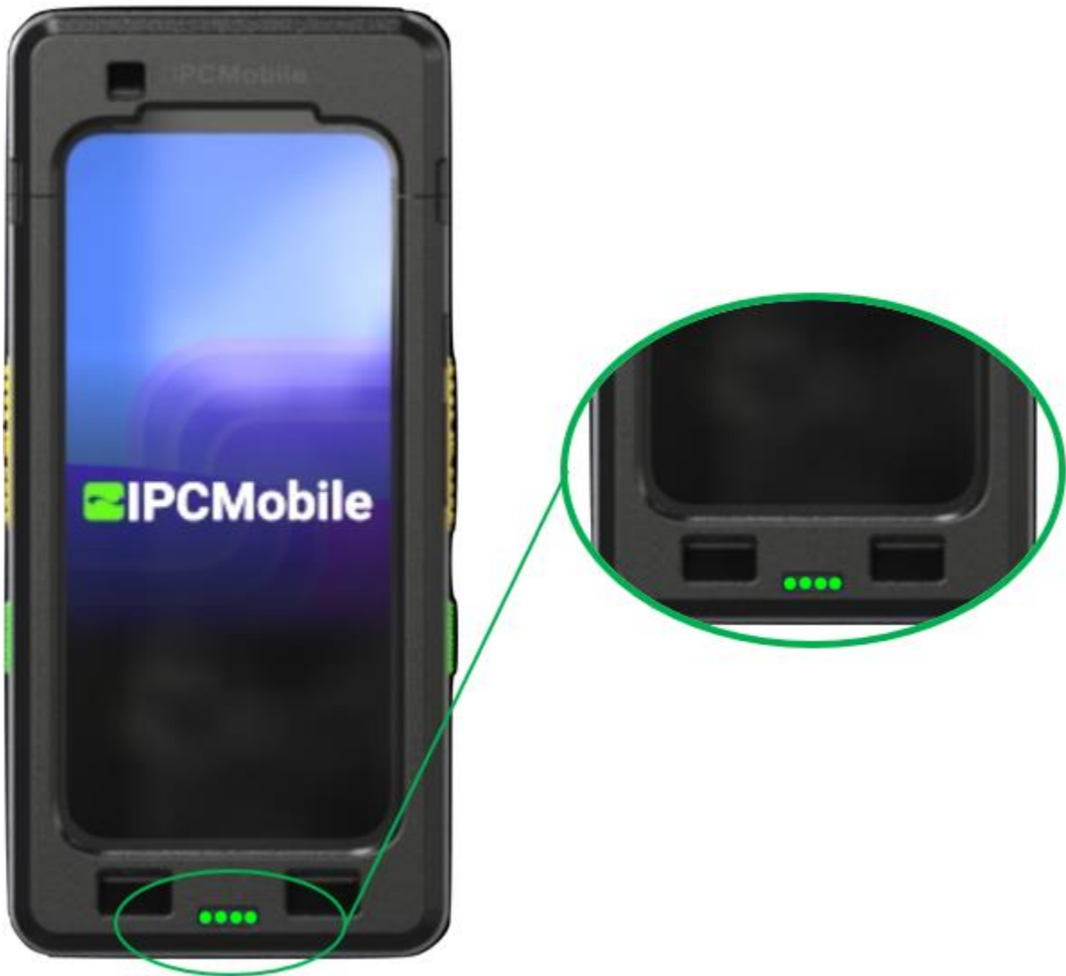
FIG. 8: LED indicators for battery percentage level
