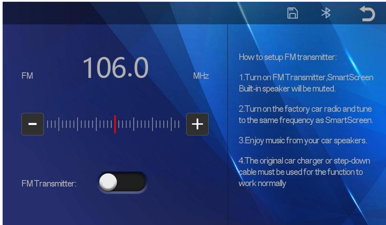
As shown in the figure, click the [FM Transmitter] button to enter the FM Transmitter function: it can emit the sound of the equipment, receive it with the original car radio, and play it through the original car horn, enjoying the original car level. When you turn on the FM Transmitter option, the monitor will no longer emit any sound. At this time, you need to turn off the FM Transmitter or match the sound to the car's builtin stereo to have sound.
