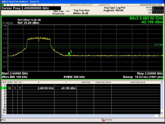
Out Of Band Emission IEEE 802.11g_Channel 11_20MHz_Antenna 0
