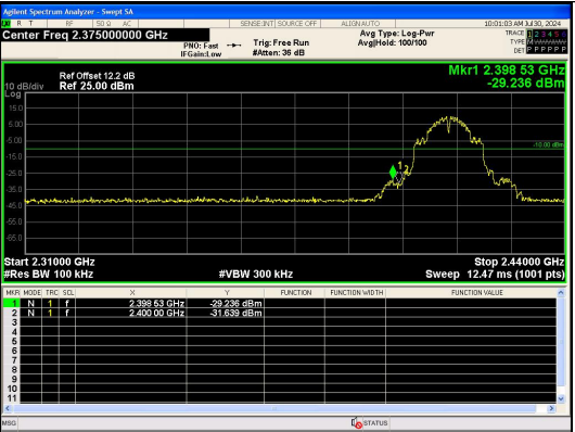
Out Of Band Emission IEEE 802.11g_Channel 1_20MHz_Antenna 0
