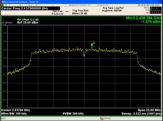
In-Band Reference Level IEEE 802.11n_Channel 6_20MHz_Antenna 0
