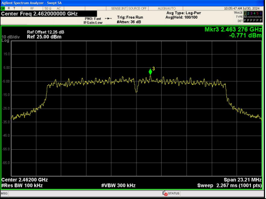
In-Band Reference Level IEEE 802.11g_Channel 11_20MHz_Antenna 0
