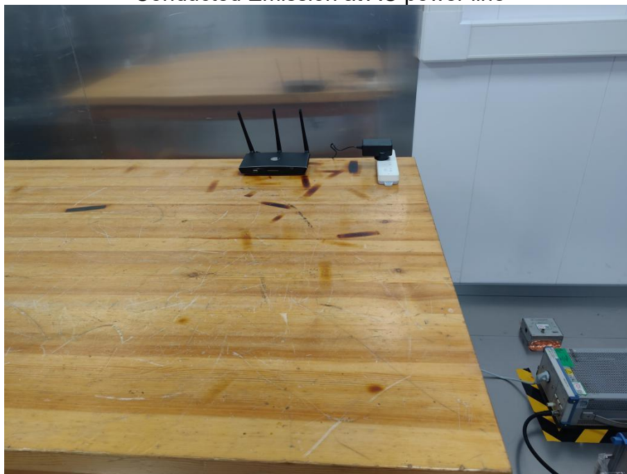
Conducted Emission at AC power line
