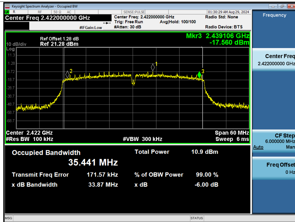
-6dB Bandwidth NVNT n40 2422MHz Ant1
