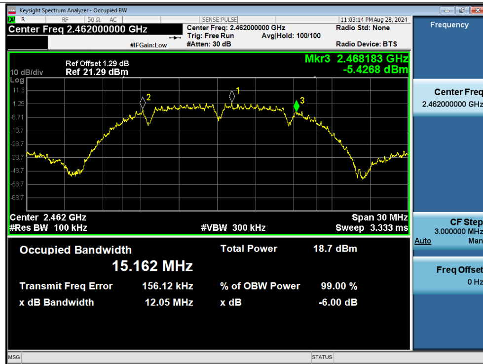
-6dB Bandwidth NVNT g 2412MHz Ant1
