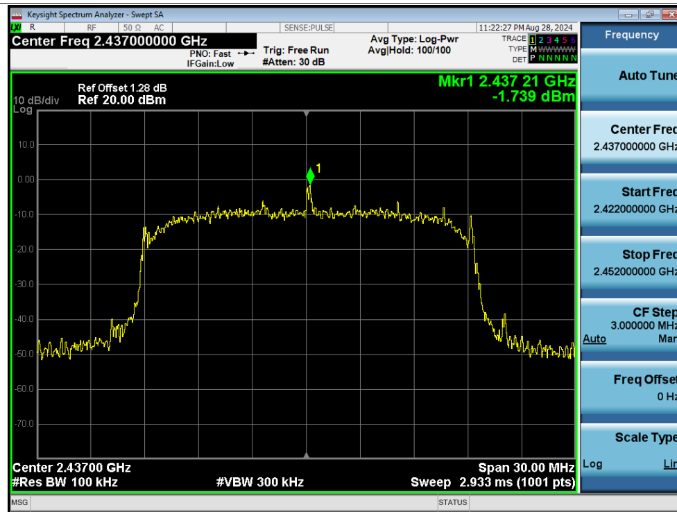
Tx. Spurious NVNT n20 2437MHz Ant1 Emission
