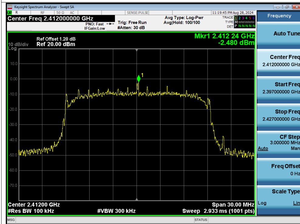
Band Edge NVNT n20 2412MHz Ant1 Emission
