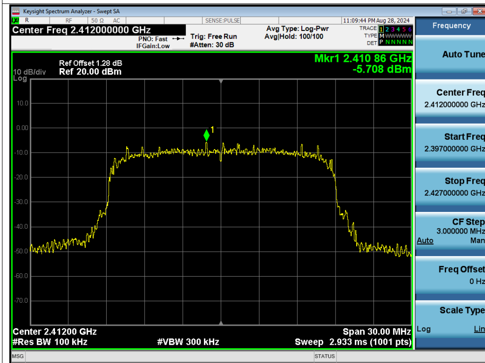
Band Edge NVNT g 2412MHz Ant1 Emission
