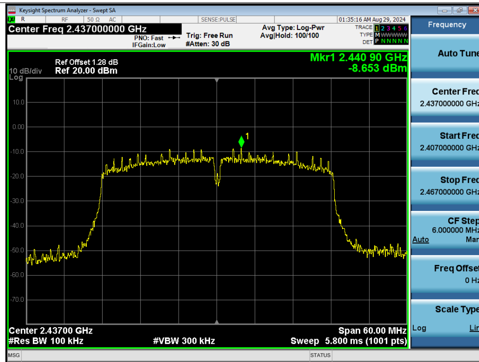
Tx. Spurious NVNT n40 2437MHz Ant1 Emission
