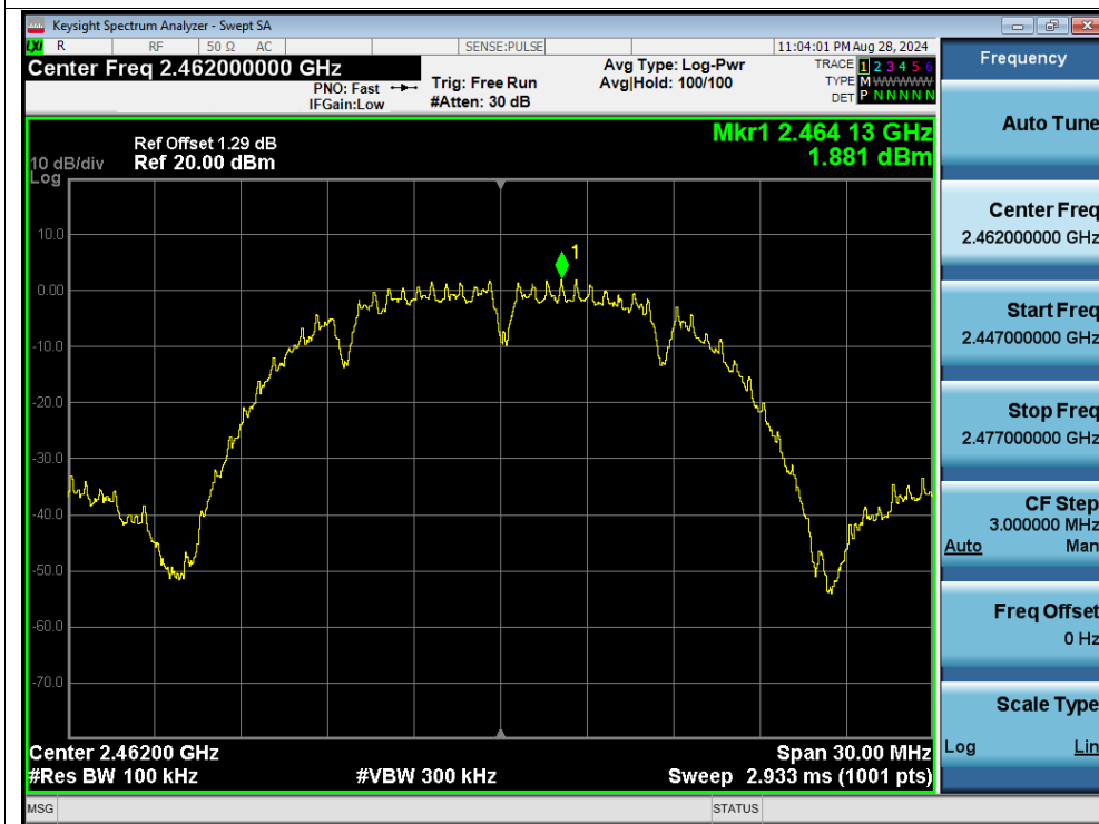
Tx. Spurious NVNT b 2462MHz Ant1 Emission
