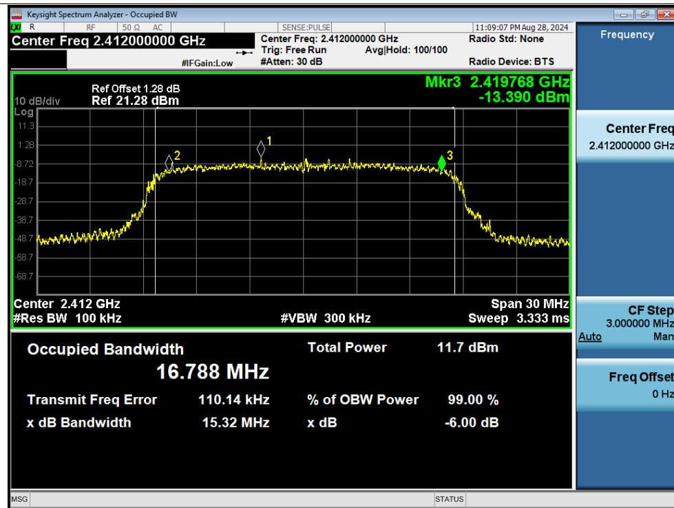
-6dB Bandwidth NVNT g 2412MHz Ant1
