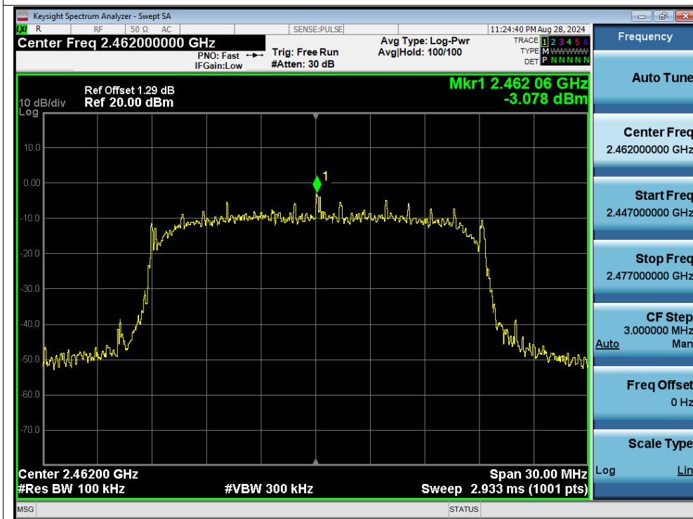
Band Edge NVNT n20 2462MHz Ant1 Emission
