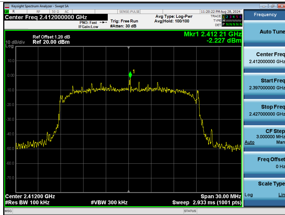
Tx. Spurious NVNT n20 2412MHz Ant1 Emission
