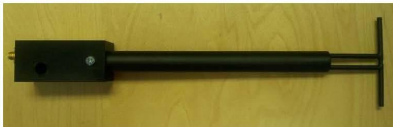
Figure 1 – MVG COMOSAR Validation Dipole
