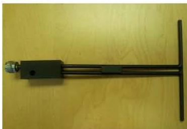
Figure 1 – MVG COMOSAR Validation Dipole
