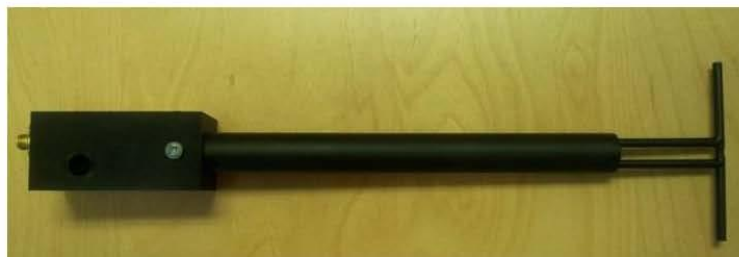
Figure 1 – MVG COMOSAR Validation Dipole
