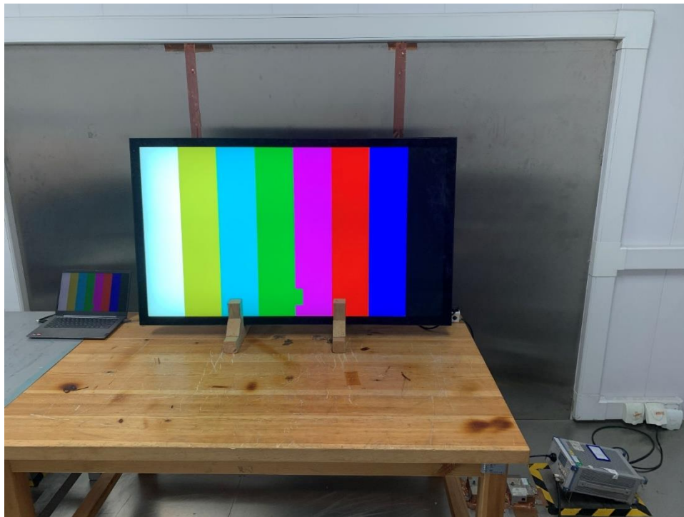
Photograph 3: Set-up for Conducted Emission on AC Mains
