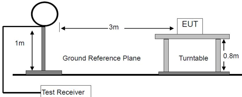
For Radiated Emission 30-1000MHz
