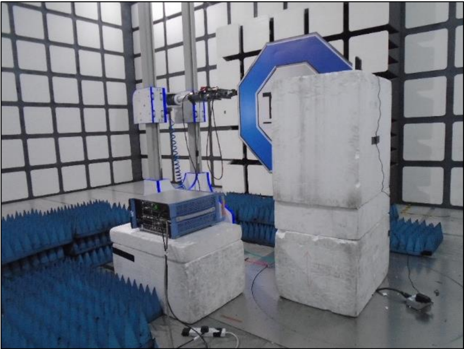
Figure 9 - Test Setup - 18 GHz to 20 GHz
