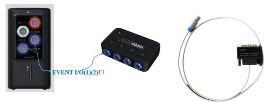
Figure 14 The TriggerIN/OUT device connects to the synchronization box via a public event forwarder
