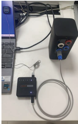
Figure 12 Schematic diagram of Light Sensor connection and use
