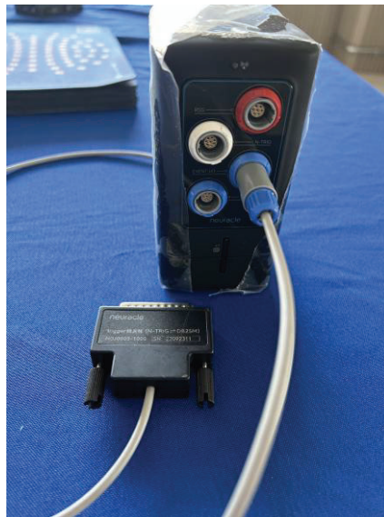
Figure 13 The TriggerIN/OUT device is directly connected to the synchronization box
