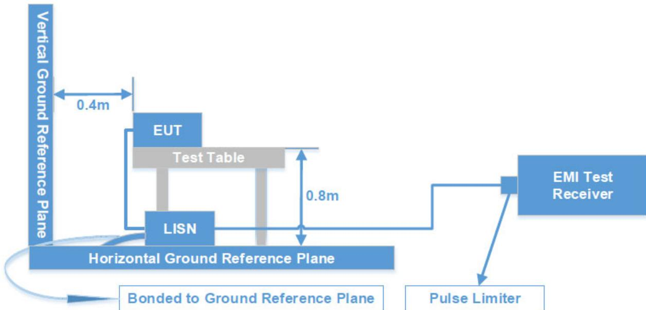
The setup of EUT is according with per ANSI C63.10-2013 measurement procedure. The specification used was with the FCC Part 15.207 limits.
