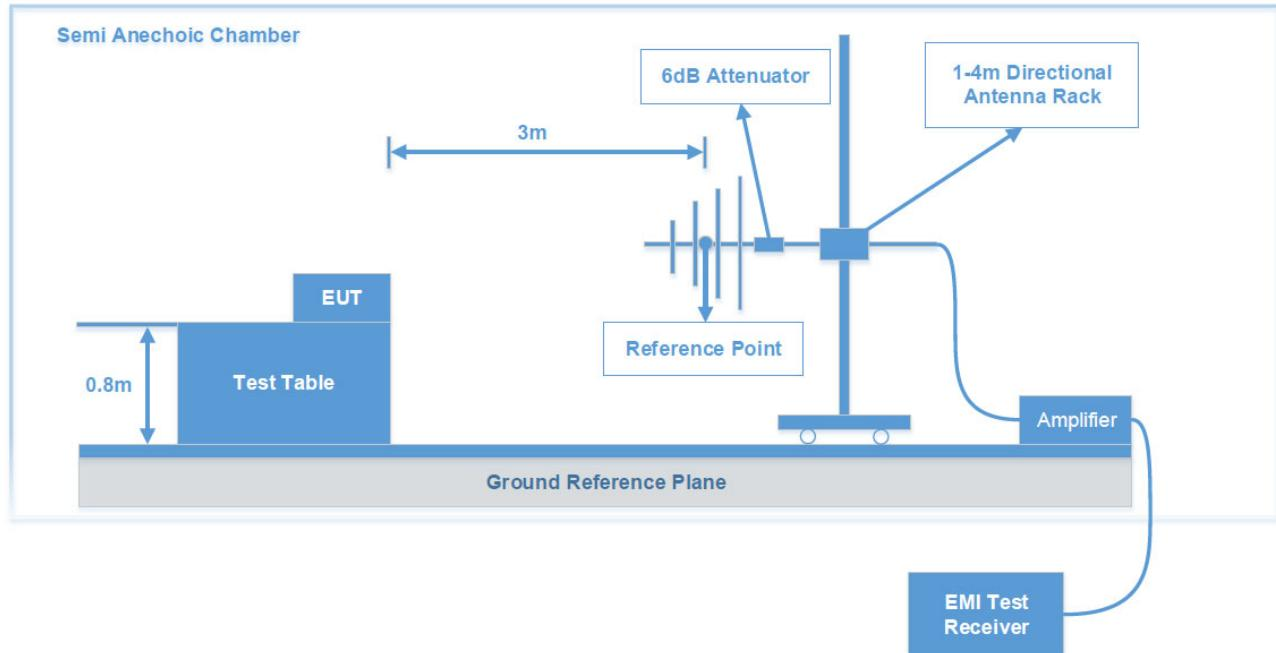
The deactivation test was performed in the 3 meters chamber test site, using the setup accordance with the ANSI C63.10- 2013. The specification used was the FCC 15.231(e) limits.
