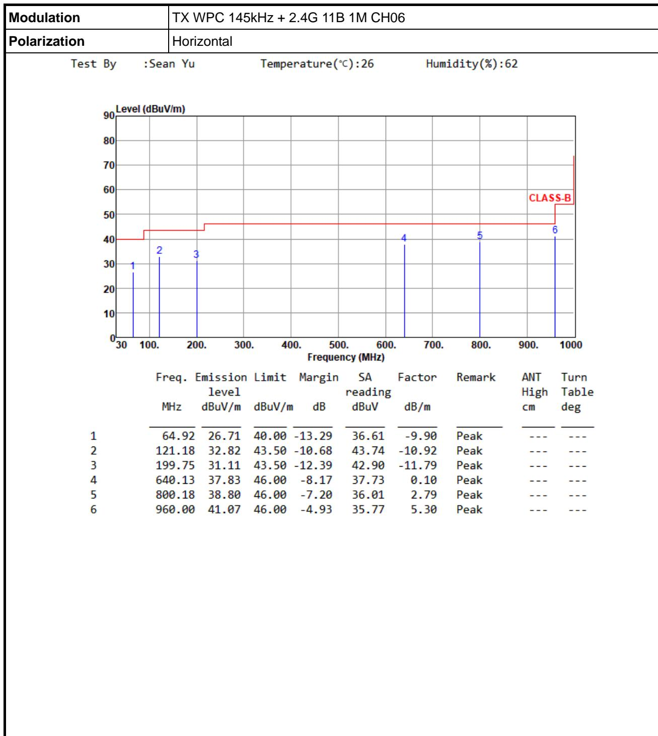
Note 1: Emission Level (dBuV/m) = SA Reading (dBuV/m) + Factor\* (dB/m)
