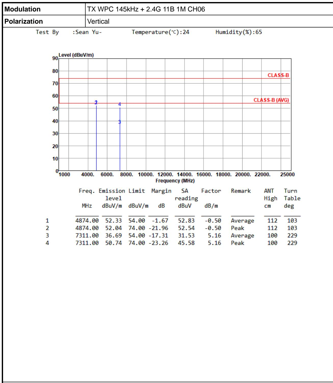
Note 1: Emission Level (dBuV/m) = SA Reading (dBuV/m) + Factor\* (dB/m)
