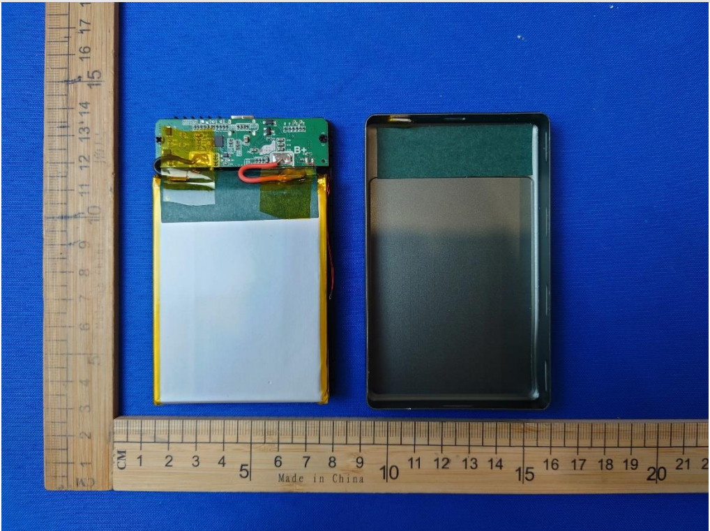
Internal View of EUT-1
