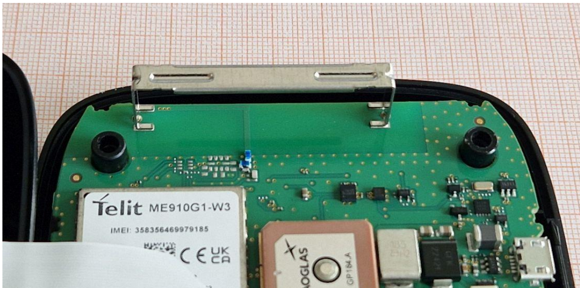
Figure 4: Close up of cellular antenna (side 1).
