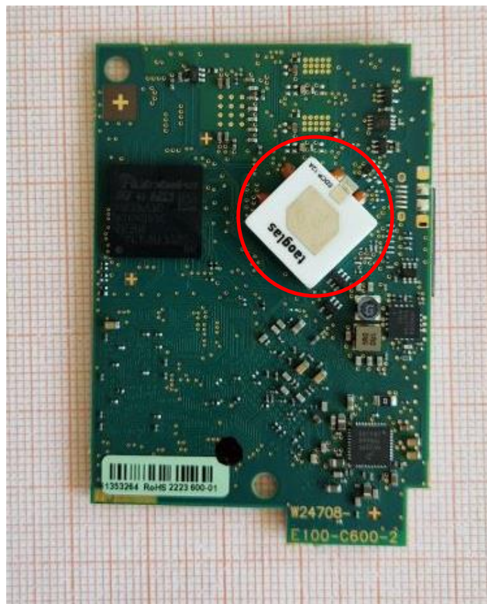
Figure 6: V2X board, with ceramic antenna
