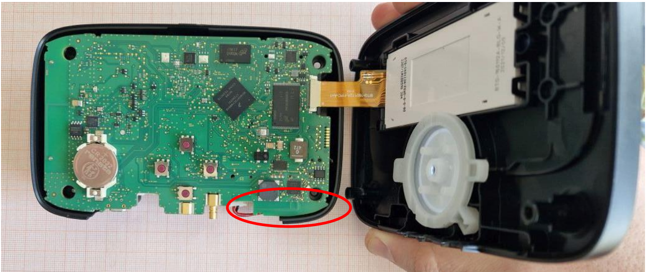
Figure 7: rear view of main board (side 2) showing 2.4 GHz antenna.
